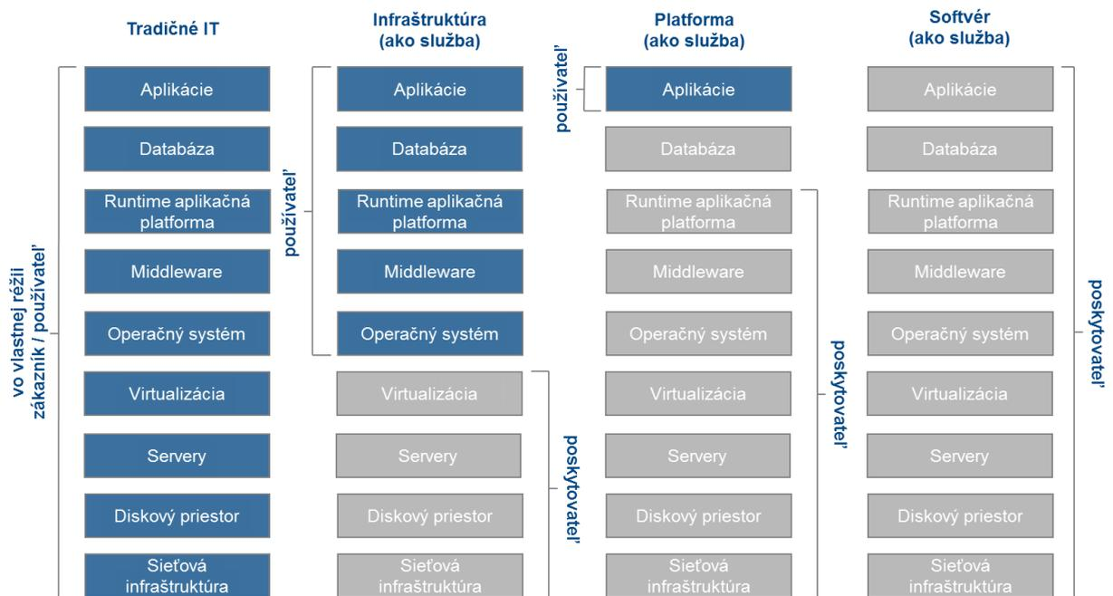
Picture 1: Control over IT services distribution between the cloud services provider and user.
